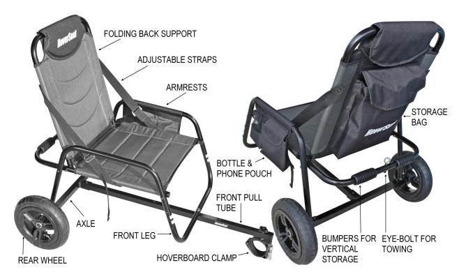
The HoverSeat XL is a light aluminum frame with a built-in folding seat that fits easily in the trunk of the car or closet or can be placed vertically against wall. When you want to use it, simply attach it to the bar in the center of your hoverboard with the specially adapted patent pending clamp, unfold chair back, and you are ready to roll!
