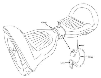
top of clamp through hole in forward pull tube and secure with provided wing nut.
