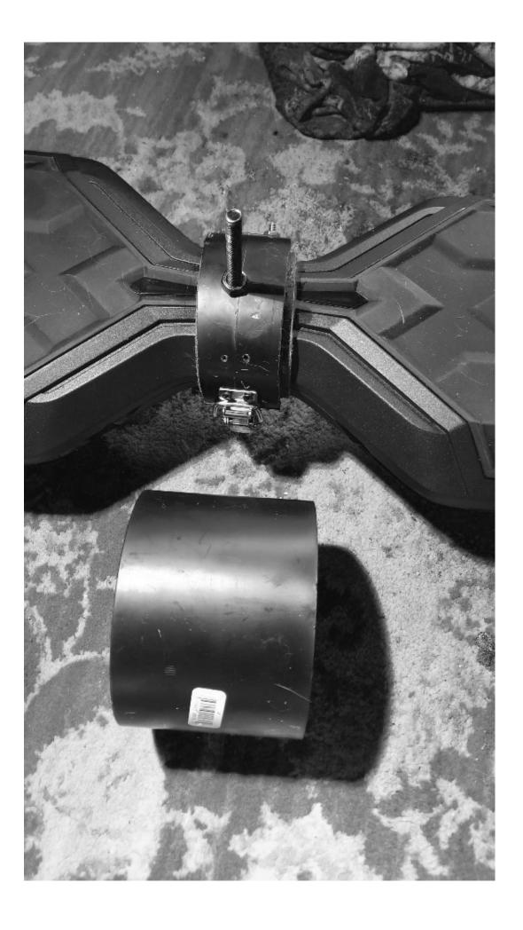
After trimmed, turn on side and cut circle in half. In one of the pieces drill a hole for the bolt in the center of the half piece. Just like the original clamp. Use a countersink drill on the inside of the hole so the panhead of the bolt is flush. Don't worry about the nut mold like the original.
