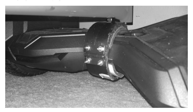
Now the other piece you mount the latch. Be sure to observe how it was mounted on original. Now attach the hinge to this piece. At this point you have a clamshell. You can use panhead bolts but our finished product will be riveted for a strong hold and smooth surfaces.
