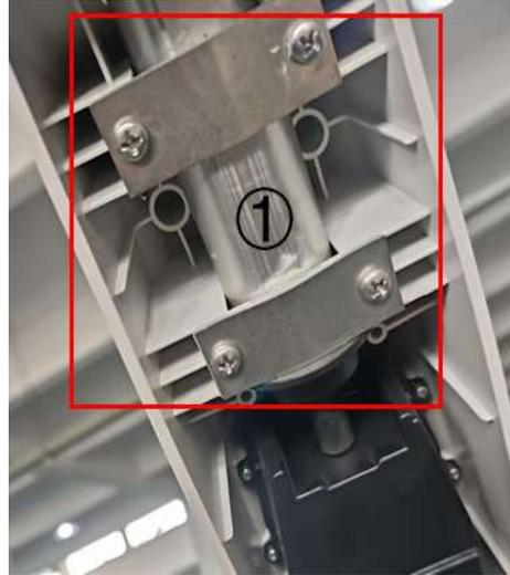
1. Check if the anti-loosening nut of the rear wiring harness is properly tightened.
