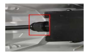
9. After securing the rear cover, tighten the anti-loosening connector of the wiring harness.
