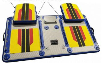
Inflate the catamaran platform to 5-10 psi or until as hard as rock using the hand pump or optional electric inflator. Use either valve and ensure pushpins are locked in the upper position.
