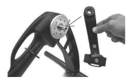
Install the Crankarm bolts; starting them by hand and then tightening to **25 ft/lbs. (35Nm)** utilizing the included 8mm hex wrench.
