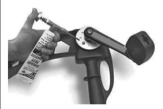
Use an extended nose grease gun to reach gears.
