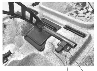
Set the aluminum thwart tube into the half round recesses located in front of the drive box. Push the slider latch forward to lock the tube in place. To remove the pedal drive push the slider latch backward to unlock the tube, repeat on opposite side.
