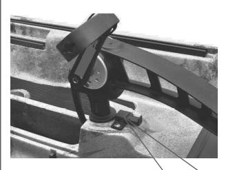
Lower the pedal drive through the drive box. Lock the pedal drive in position with the slider latch installed on the front of your drive box. Replace the drive box cover.
