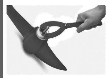
Remove the propeller by following the "Shear Pin Replacement" instructions on the facing page. Next, remove the cartridge using a spanner wrench with 3/16" pins.
