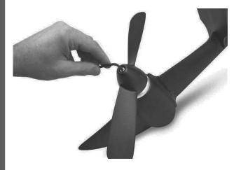
Remove the end bolt using a 4mm hex wrench. Pull the prop straight back to remove the prop and expose the shear pin.
