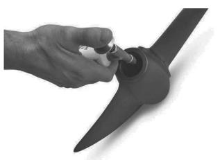
Grease the Lower Transmission Gear by inserting the extended nose grease gun and injecting 2 pumps onto the gear.
