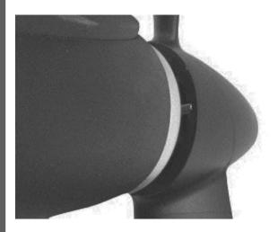
Replace the prop, making sure the pin sets into recesses the in prop. Replace the bolt and tighten 1/2 turn past the bolt engagement with the propeller.
