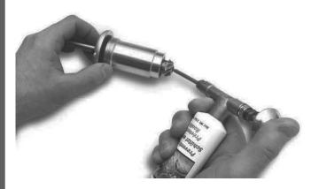
Grease the Propeller Gear on the cartridge with 2 pumps from the grease gun.
