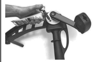
Inject 2 to 3 pumps of grease and replace grease port screw. Rotate crank arms slowly to apply grease throughout the gear assembly.
