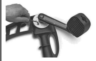
Remove grease port screw using a 3/16" hex wrench.
