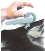
12. Insert wrench and begin turning right. Hold back female valve with back hand by pinching in on the tube.
