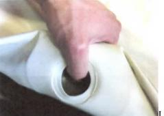
10. Lineup inside female version of the valve so that it is evenly located around the hole. There should be several mm of extra fabric on each side of the hole (Top, Left, Right, and Bottom).
