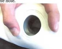
8. Once male valve end has been removed, move boat and find the back female version of the valve located inside the tube.
