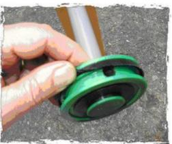
On the end of the plunger you will see 3 ridges: A top ridge, a 2nd ridge that is just below the top one, and a bottom ridge. When the black rubber seal is properly installed it is in the valley between the top ridge and the 2nd ridge, and it covers the 2nd ridge. Photo shows proper location and orientation of the black rubber seal.
