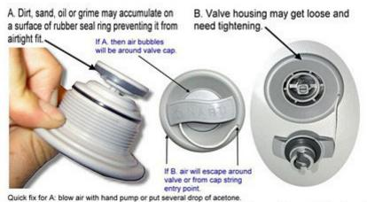
Quick fix for B: tighten valve with a special tool, or apply household sealant around valve and inside string entry point.
