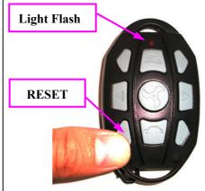
In order to save the battery power. Press the "RESET" (red light flash) to turn the remote controller into a sleep mode.
