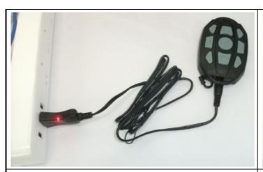
Charge the remote controller before first use. Connect the USB cable to the remote controller and the power source.
