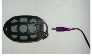
**3.** Disconnect the remote controller from the USB cable. ( the remote controller is now activated and is also power consuming)
