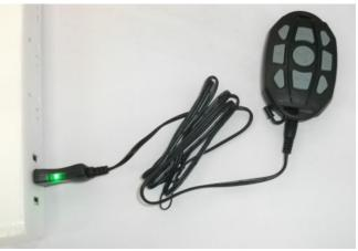
When the USB cable light turn green indicate the recharge is completed.
