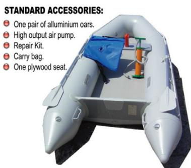
All boats are made of 1,100 Dtex high strength fabrics consisting of 5-layer thick construction and double bonded seams. One layer Neoprene, two layers of Nylon, and two layers of PVC fabric for outer strength and an excellent deterrent of ultra-violet rays.
