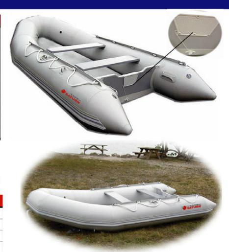
12.6-feet SD385 is one of the largest SATURN inflatable boats available. SD385 is great as a fishing boat or as large dinghy to carry up to 7 person maximum. SD385 boat made of 1,100 Dtex High Strength fabric consisting of 5-layer thick construction and double bonded seams. One layer Neoprene, two layers of Nylon, two layers of Strongan fabric for outer strength and an excellent deterrent of ultra-violet rays.
